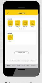
7. Long press the daylight sensor and link it to the group of 1-10V dimmers for that circuit. Tap on OUTPUT LEVEL to set the target light level.
