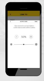
8. Using your light meter, set your desired light level target and tap SAVE. The light level output is now controlled automatically based on the set target (ON/OFF control from hardwired wall switch).
