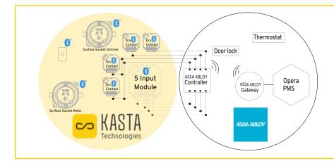
> KASTA 5 Input Module and ASSA ABLOY set the mode of the room based on the inputs from PMS, Door Lock and Motion Sensor.
